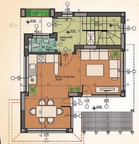
VILLA NOVA FLOOR PLAN ±0.00 Unfolded built up area for Level 1 = 47.9m 2 Unfolded built up area for Level 2 = 58.2m 2 Total unfolded built up area of the house = 106.1m 2 The house is suitable for a plot with an entrance, situated on the left side
