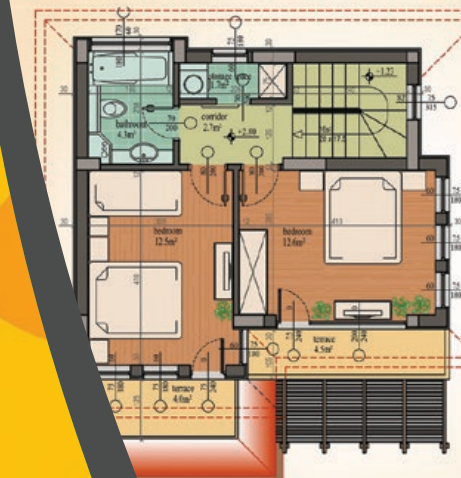
VILLA NOVA FLOOR PLAN +2.80 Unfolded built up area for Level 1 = 47.9m 2 Unfolded built up area for Level 2 = 58.2m 2 Total unfolded built up area of the house = 106.1m 2 The house is suitable for a plot with an entrance, situated on the left side
